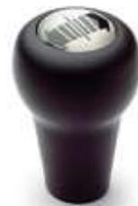
Knobs with electric components are assembled with dust-proof pushbuttons with 5 A resistive (3 A inductive) maximum current, maximum voltage 28 VDC, 2 or 4 pins and protection degree IP64 (IP68 on request). Pushbuttons serviceable plastic cap actuator available in 9 different colours and flush or raised shape.
